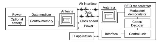
Figure 3. The working principle of RFID
